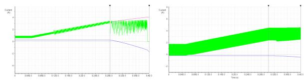
V<sub>IN</sub> = 6V: I<sub>L1</sub> 峰值 = 3.37A, I<sub>LOAD</sub> = 3.17A
